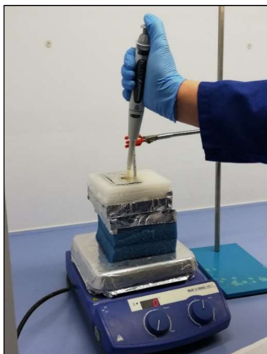
Figure 3.2. Injection of oxidizer into coffee-cup calorimeter
